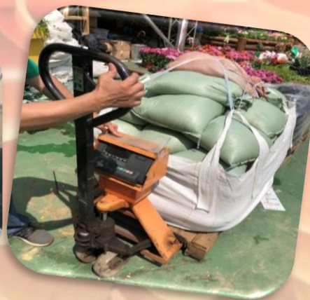
Pallet truck (with built-in electronic scale)
